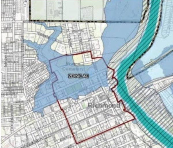
The proposed raising and reconstruction of 2nd Street in Downtown Richmond has the potential to remove a portion of the district out of the flood hazard area.
